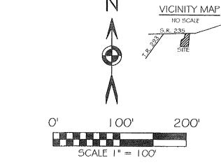
BASIS OF BEARING: BEARINGS ARE BASED UPON THE OHIO DEPARTMENT OF TRANSPORTATION V.R.S. NAD 83(2011). OHIO STATE PLANE NORTH ZONE 3041. GEIOD 12A GROUND DISTANCES USED.
