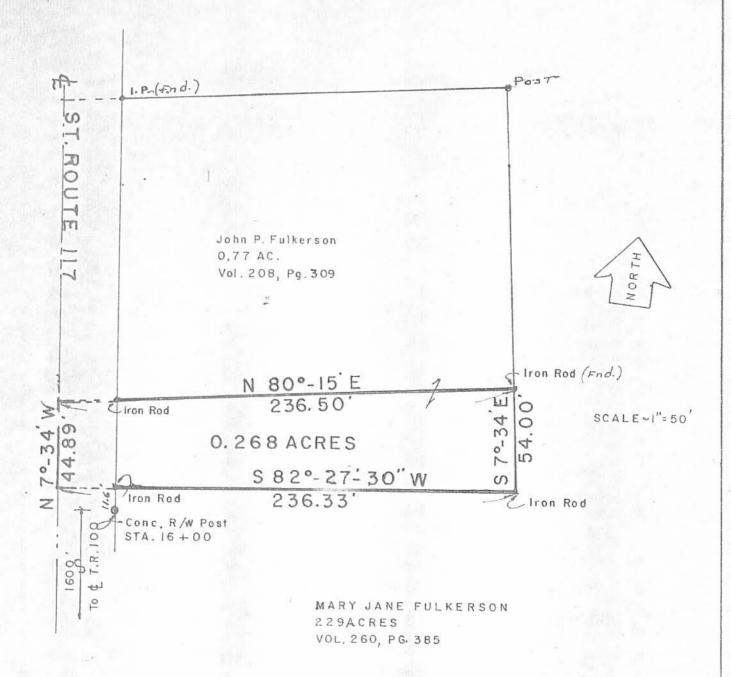
SURVEY OF 0.268 AC. ADDITION TO THE JOHN P. FULKERSON 0.77AC. (Vol.208, Pg. 309) V. M.S. 9949, RICHLAND TWP, LOGAN CO., OHIO
