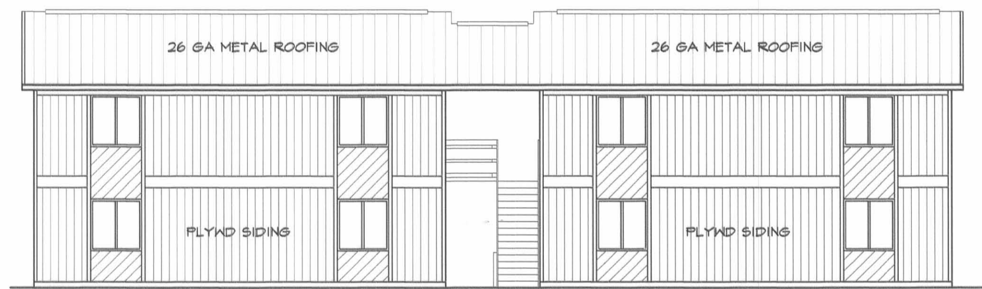
PARKING SIDE ELEVATION REAR
