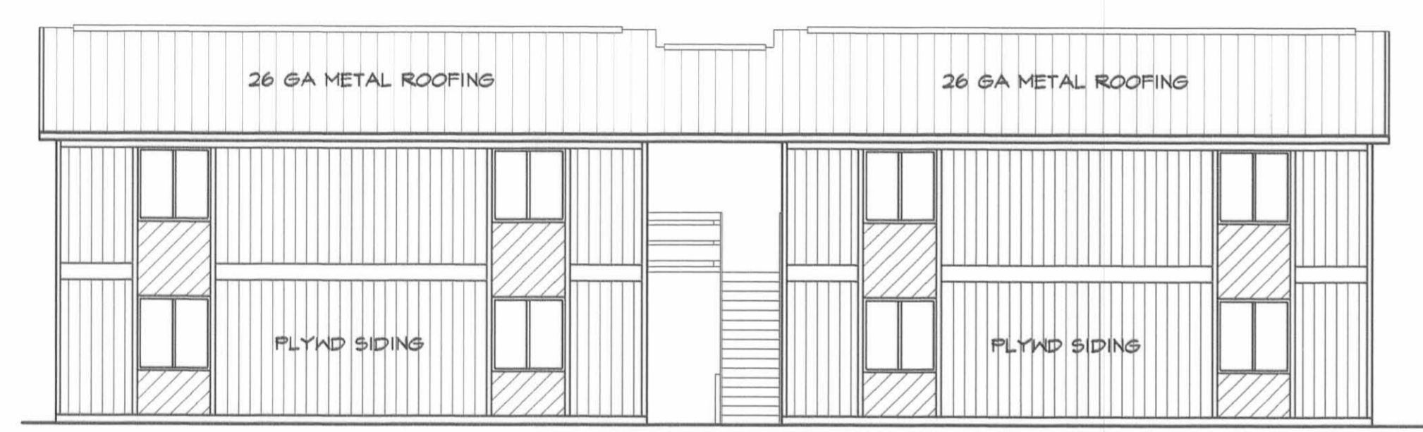
PARKING SIDE ELEVATION REAR
